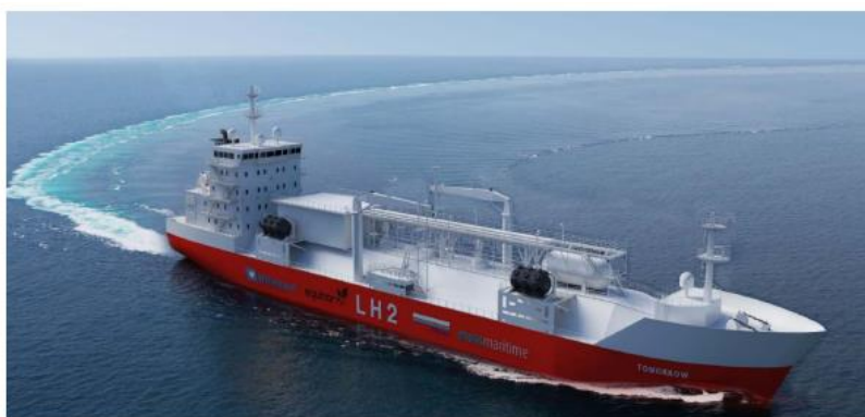
Figure 9: Conceptual design of a liquid hydrogen bunker ship /7/.
